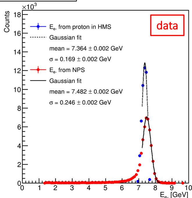
Energy resolution in the calorimeter
