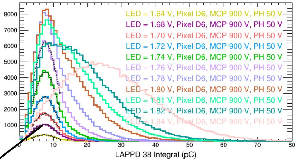
→ Each distribution of charge integral corresponds to a fixed LED voltage and a fixed number of triggers
