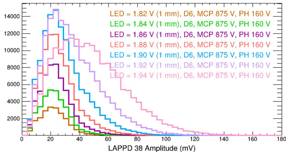
Single photoelectron distributions obtained from LAPPD 38 at a MCP voltage of 875 V and a photocathode voltage of 160 V with LED photons collimated through a 1 mm hole
