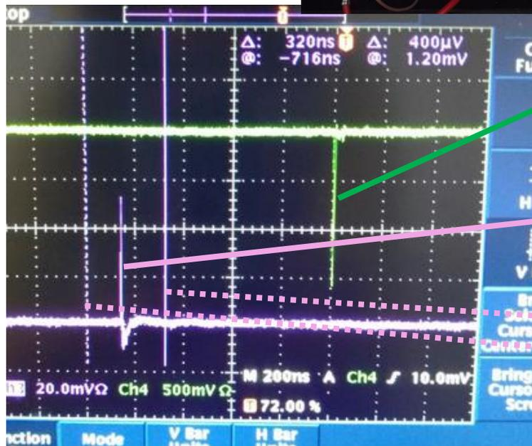
Trigger: pulse that drives LED
