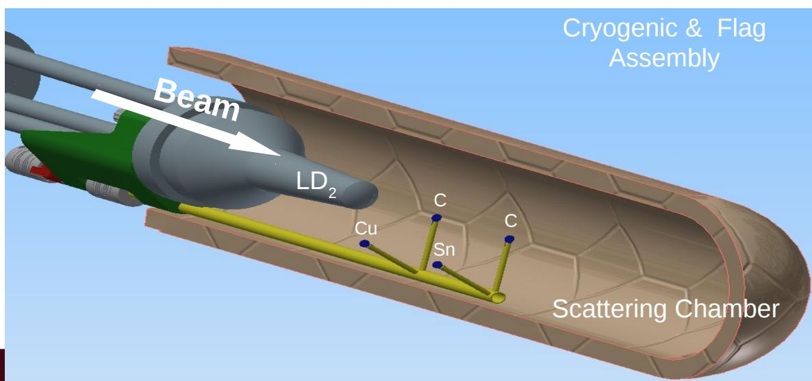
Newly built Hall B cryogenic target;
