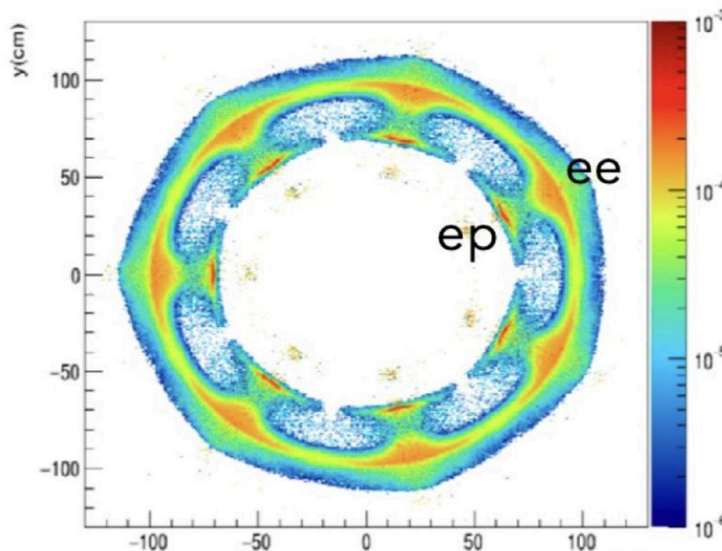
Radial distribution at detector plane 26.5 m from target
