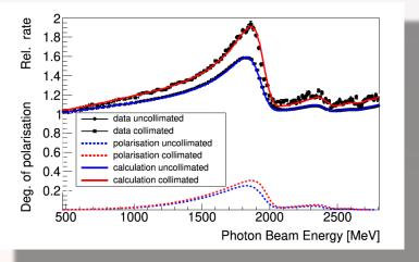
*Diamond* Radiator  $\rightarrow$  Coherent Bremss  $\rightarrow$  Linearly Polarized  $\gamma$  beam
