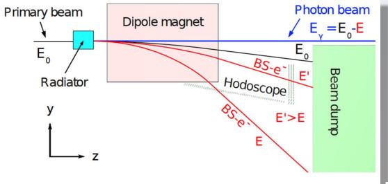
linearly polarised photon beams generated by coherent bremsstrahlung using a diamond crystal radiator.
