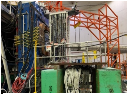
Test of SBS GEMs during 3He GEN.
