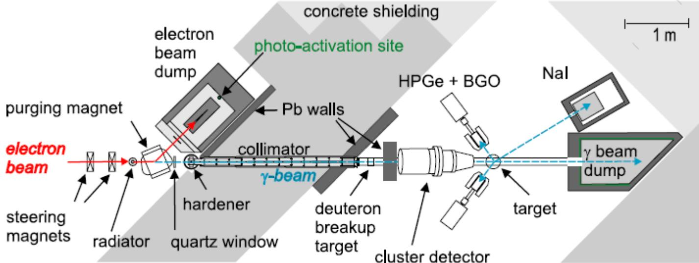
**Figure 1.** Bremsstrahlung facility and experimental area for photon-scattering and photo-dissociation experiments at the ELBE accelerator.
