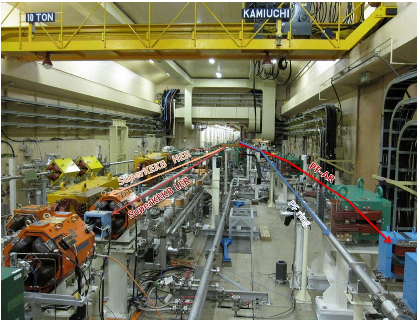
Simultaneous Top-Up Injection into four Rings+ Damping Ring
