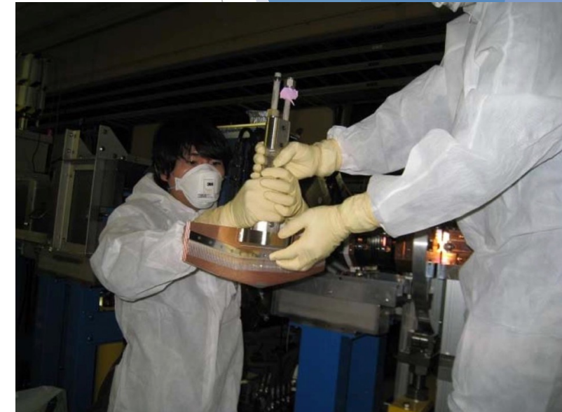
Replacing the damaged and radiated collimator
