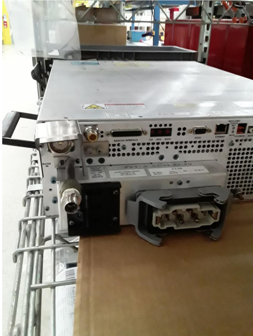
Fig.6. RF generator (MKS Sure Power QL6513A-OF03) at frequency 13.56 MHz and power up to 6.5kW.
