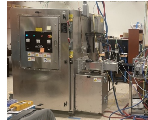
Modified Industrial 915 MHz magnetron RF source
