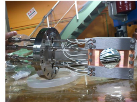
Water-cooled baffle type current detector 500 W max. for each side
