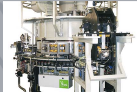
The IBA rhodotron – a commercial accelerator used for e-beam sterilization
