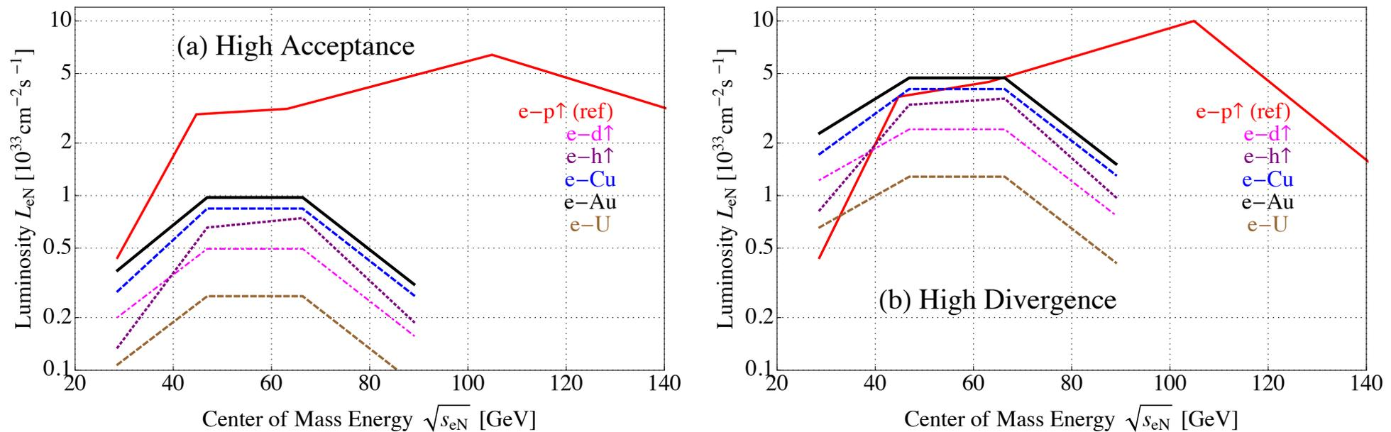
Figure 1: EIC  $e$ - $A$  luminosity  $L_{eN}$  for  $N = p, d, h, Cu, Au$  and  $U$  beams, all with Strong Hadron Cooling. Part (a) shows the luminosities for the High Acceptance limits imposed on the angular beam spreads  $\sigma'_{A,x,y,max}$  at the Interaction Point (Table 2), and part (b) for the High Divergence limits. With Strong Hadron Cooling the peak and average store luminosity are close. The  $e$ - $p$  reference case data are taken from Ref. [1].
