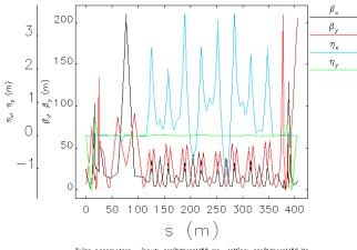
Twiss parameters——input: arc2ldzeroM56.ele lattice: arc2ldzeroM56.lte
