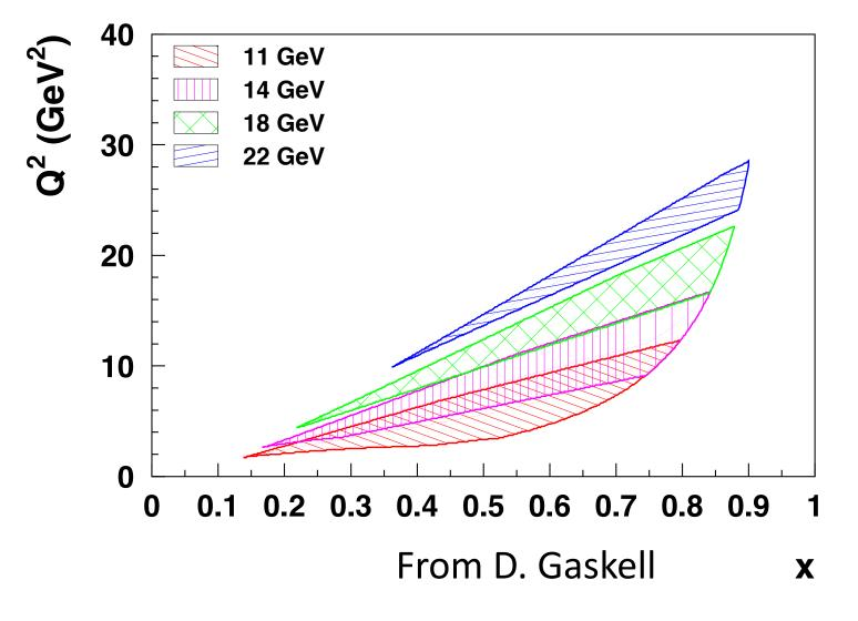
Kinematic ranges accessible in Hall C with existing HMS and SHMS spectrometers and that can achieve two  $\varepsilon$  values separated by 0.2 with a minimum  $\varepsilon$  of 0.1
