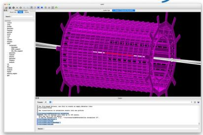
Screenshot of eAST GUI with geometry of Beam pipe, DIRC and EM\_CAL supports @IP6 / Athena. Three GDML files of these structures are loaded separately and combined in eAST.
