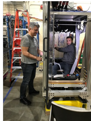
Miktat Imre and Carlos Domingues installing PMT/bases assemblies
