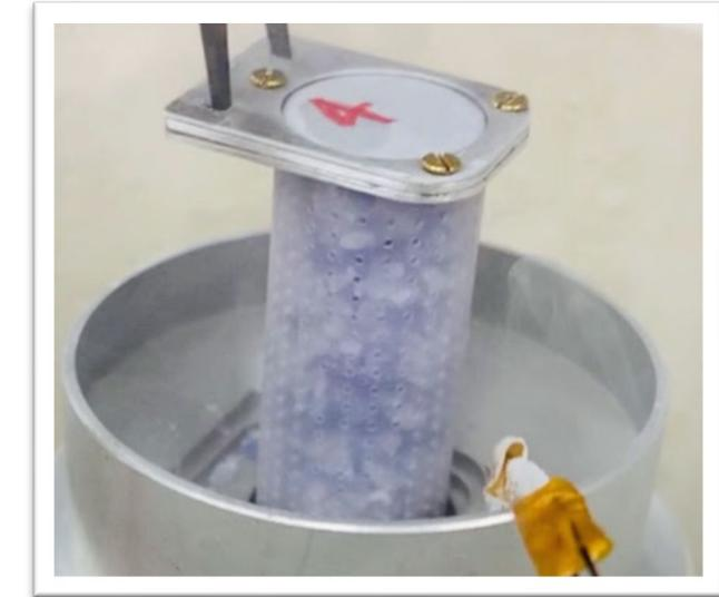
Solid target cells kept in 80K liquid Argon bath (Ammonia freezes at 195.5K)
