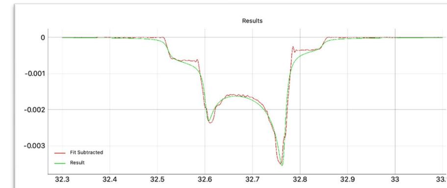
NMR software measuring  $d$  polarization
