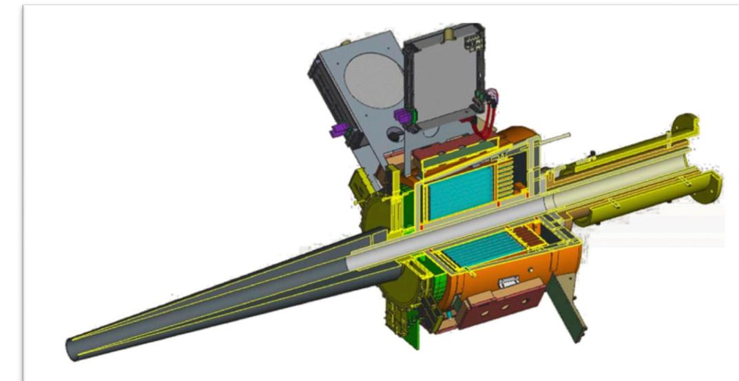
(Bottom) Schematic of the CLAS12 forward tagger
