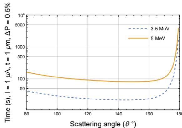
Measurement time required for corresponding angles.
