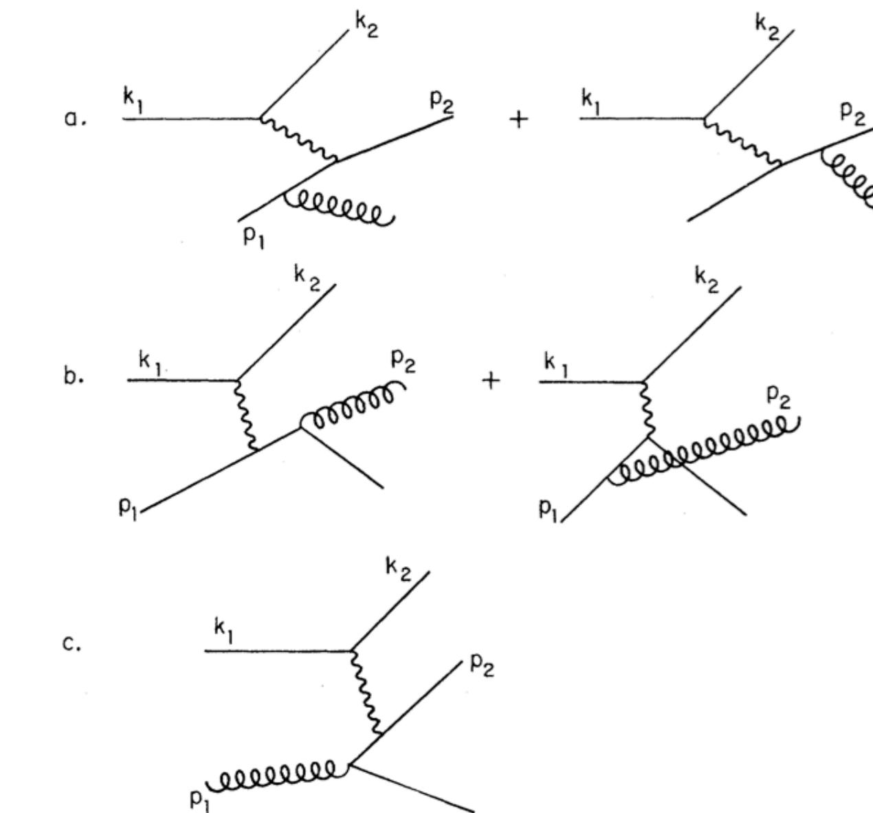
FIG. 1. Diagrams contributing to semi-inclusive  $\mu$ -parton scattering to first order in  $\alpha_s$ .  $k$  ( $p$ ) denotes muon (parton) momentum. The wavy line is a virtual photon. The curly line is a gluon.
