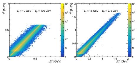
Muon (and electron) pair  $p_T$  will provide an excellent calibration tool for the direct proton  $p_T$  measurement; possibly, also the proton acceptance can be well calibrated using the exclusive muon pairs
