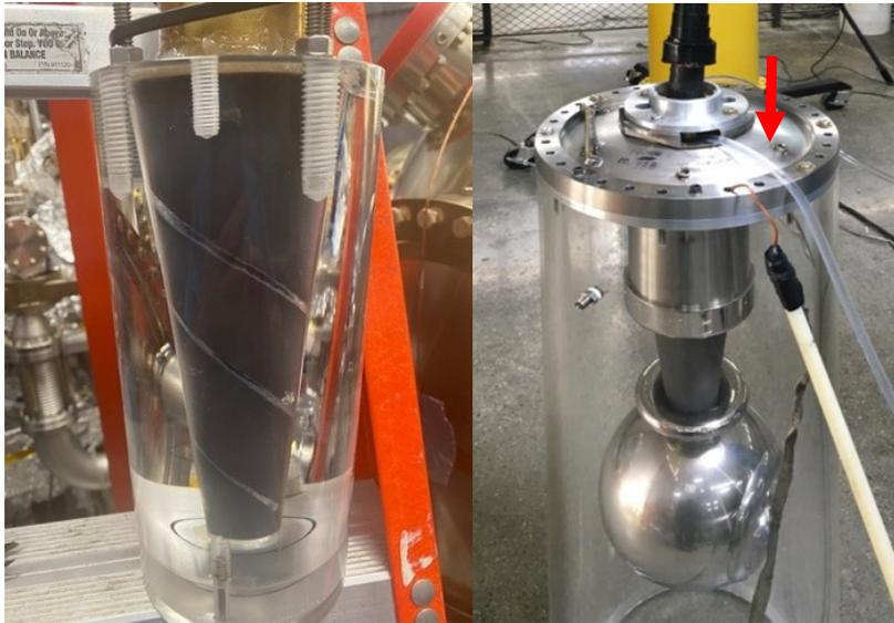
Customer designed HV plug with cooling channel
