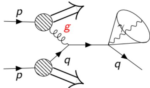
$$r_{\text{cone}} = \sqrt{(\delta\eta)^2 + (\delta\phi)^2} = 0.5$$
