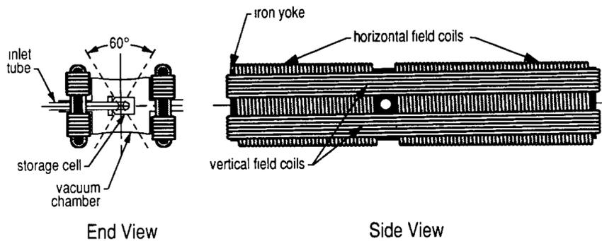
Open magnet for a long cell target
