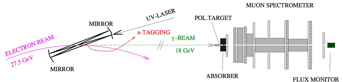
Figure 4: The basic layout of the APOLLON experiment. A laser beam is brought into collision with the HERA electron beam. The Compton backscattered high energy photons produce  $J/\psi$  mesons in a polarized target. The energy of the photons is selected by tagging the recoil electrons.
