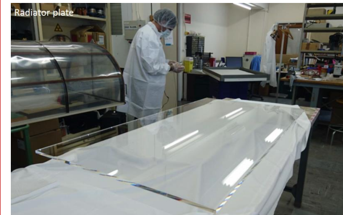
10 mm-thick LHCb TORCH prototype
