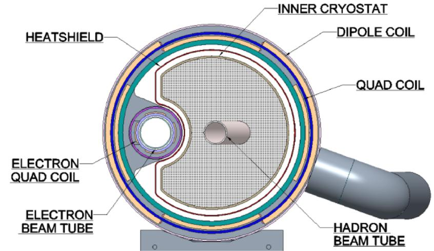
Figure 3.4: Cutaway view of the B0 spectrometer with warm space for detector elements highlighted in the cross hatch region. The view is from the IP end of the magnet with the electron beam pipe on the left and the hadron beam pipe on the right. As described in the text, B0 uses a combination of superconducting coils to provide pure focusing (with zero dipole field) at the electron beam and a 1.3T average magnetic spectrometer field at the hadron beam.
