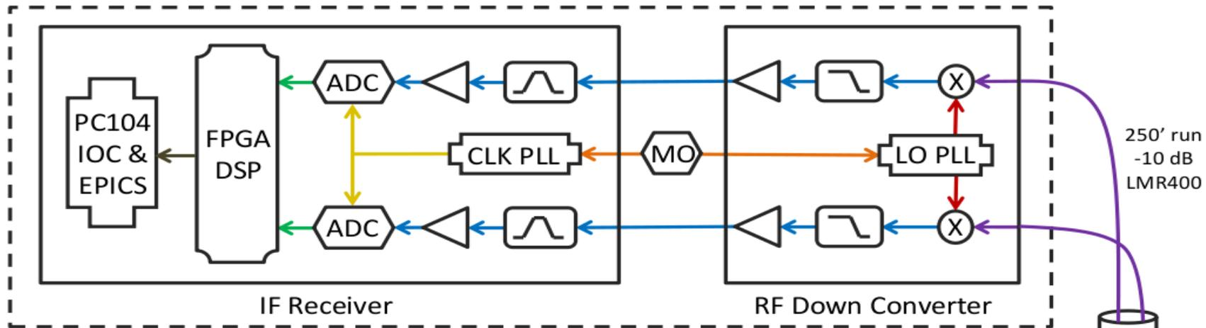
FPGA filters and provides channel waveforms to EPICS
