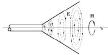
Surface wave evolution inside the launcher
