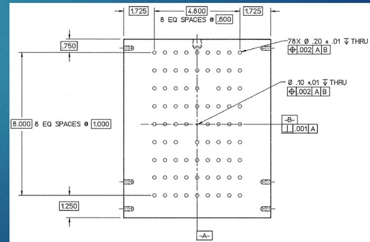
HMS Sieve Slit Schematic
