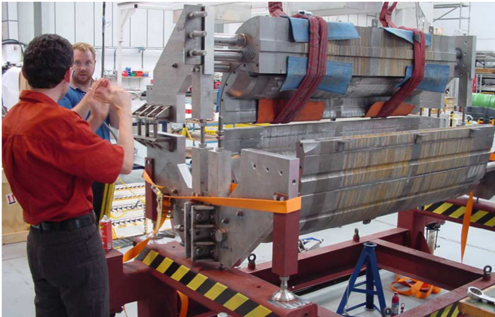
Hall C Q1 Yoke fit-up in cold mass assembly jig.
