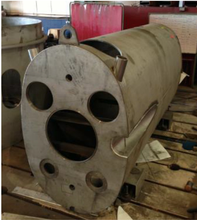
Hall C Q1 Outer Vacuum Cryostat weldment showing beamline cutout at mid-plane.
