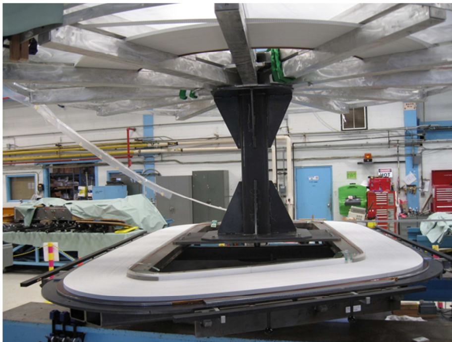
Hall B Torus: The first pancake winding complete.
