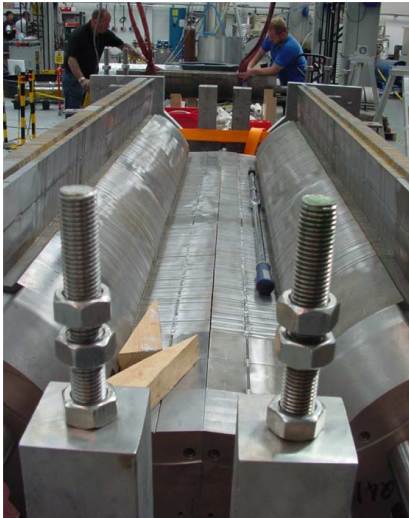
Hall C Q1 lower half yoke fit-up in cold mass assembly jig.
