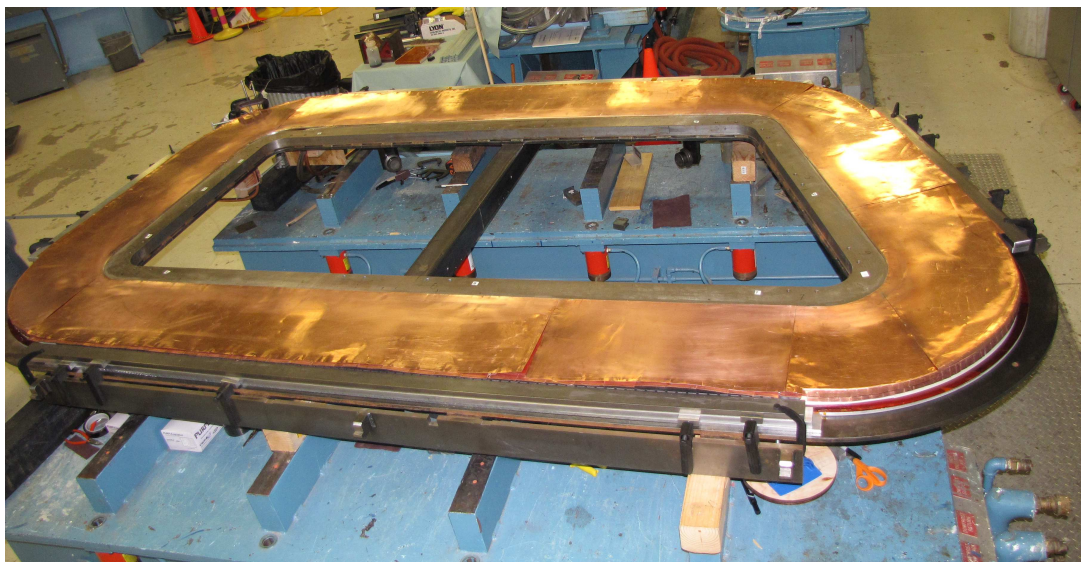
Prototype Hall B Torus Coil at FNAL with copper “thermal drain” sheets installed.
