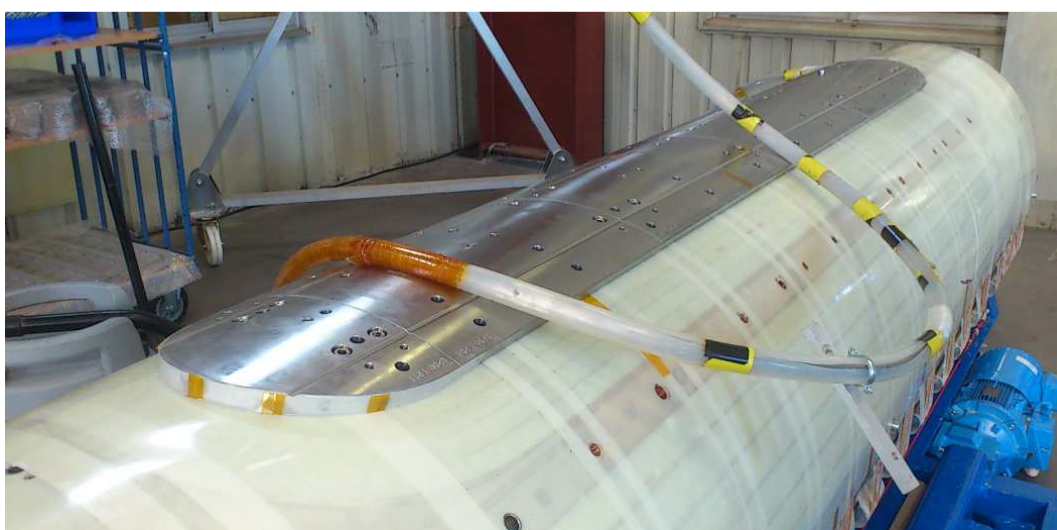
The start of the second layer winding for the Hall C Dipole prototype. The G10 ground insulation layer is strapped in place over the first layer.
