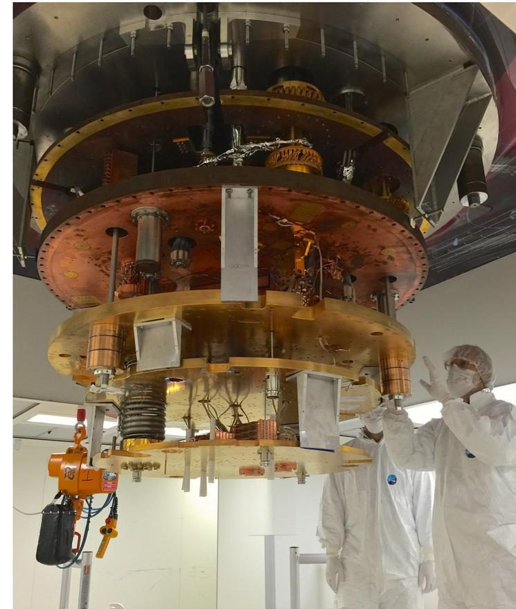
A Leiden Cryogenics DR cools the 1 ton CUORE neutrinoless double beta decay detector to 10 mK.
