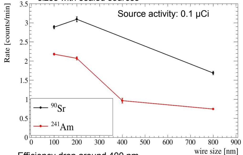
Efficiency drop around 400 nm.
