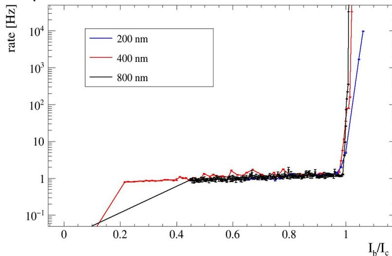
Limited by noise/interference at low bias currents  $\rightarrow$  working to improve the SNR in this region
