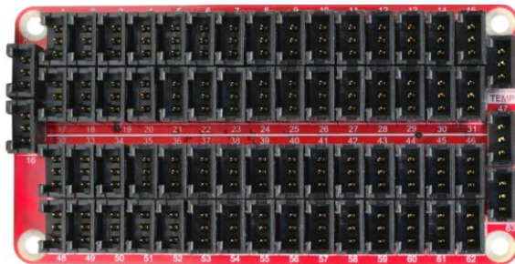
A5253: sparse SiPM cabling
