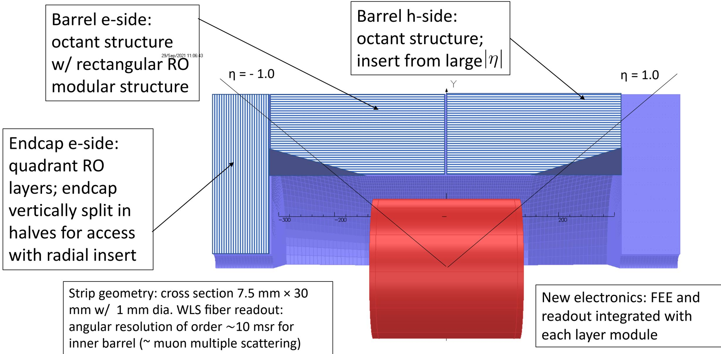
N.B.: maximum scintillator readout strip length  $< \sim 3$ m in all layers
