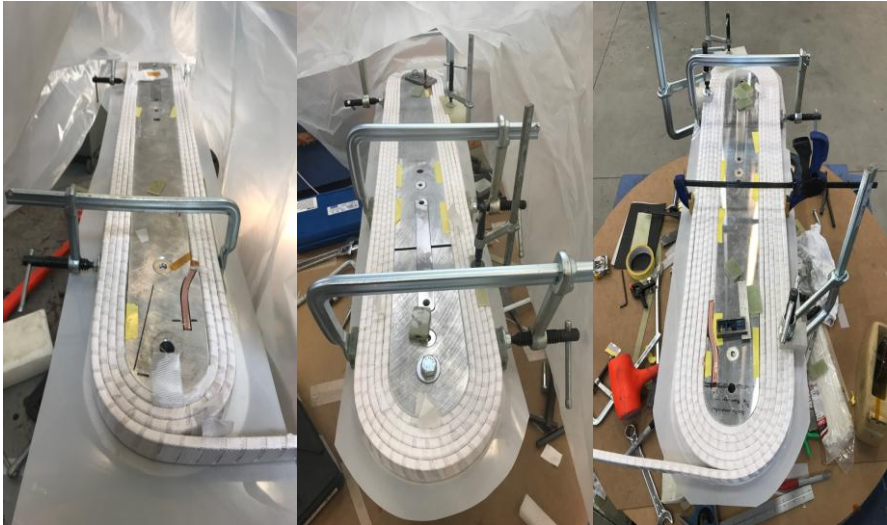
Sub-coil 1, 2 and 3 after winding
