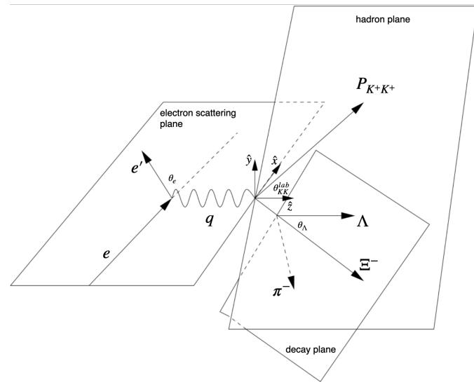
Lab frame for hadron reaction and decay planes
