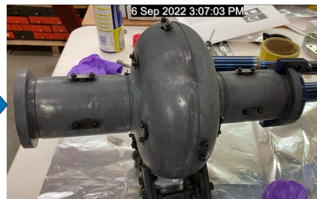
After heating at 700 C under vacuum
