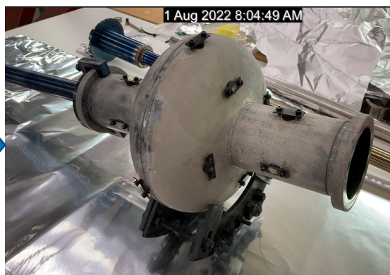
After B-Mg reaction in Ar at 700 C (furnace)
