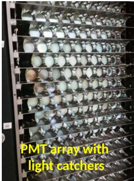
[3] PMTs as seen from inside the GRINCH.
