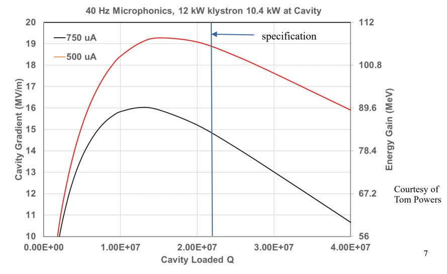
C100 RF Power Limited Gradient as a Function of Loaded-Q
