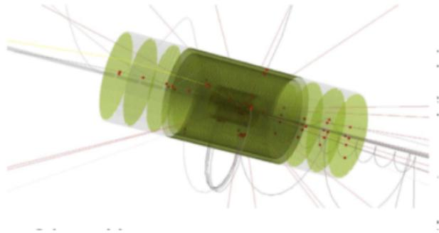
Figure 8: Silicon tracker 3D-schematics. The tracker consists of six cylindrical barrel layers covering the central region, and six tapered disks each in the forward and backward region.
