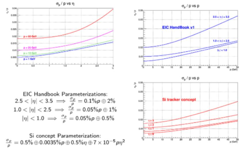
Figure 10: Momentum resolutions from the parameterization versus  $\eta$  (top-left), versus particle momentum for Handbook parameterization (top-right), and for the Silicon tracker concept (bottom right). The Handbook values are presented at bottom-left.
