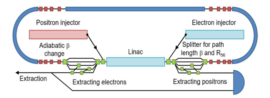
Space for up to three positron injectors and one chopped electron injector inside ring. To reduce systematics, positron injectors might be configured to select either positrons or electrons from pair production
