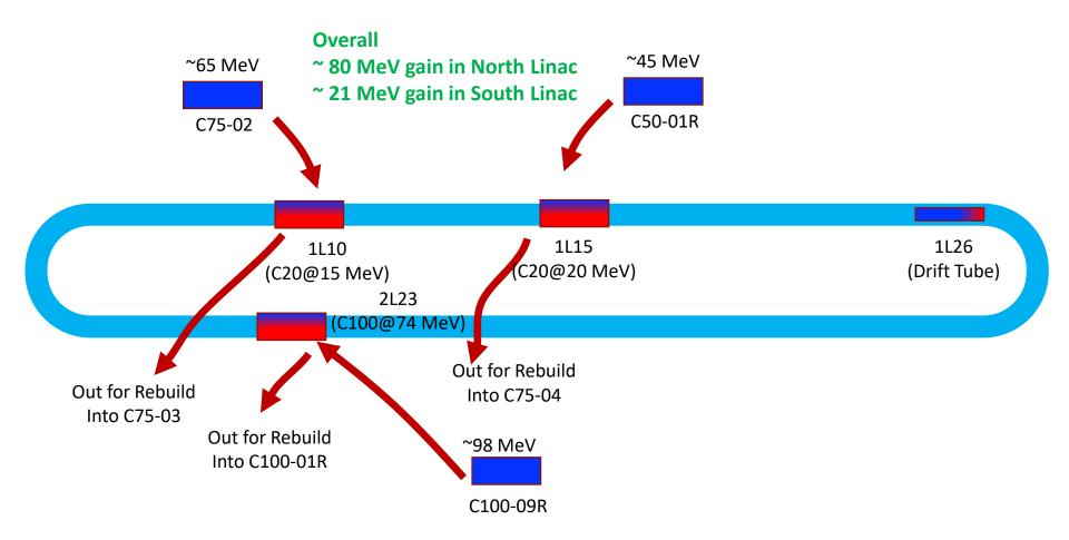
December forecast. The situation is in flux and plan will be adjusted as one becomes aware of the SRF reach (affected by component failures, etc..)
