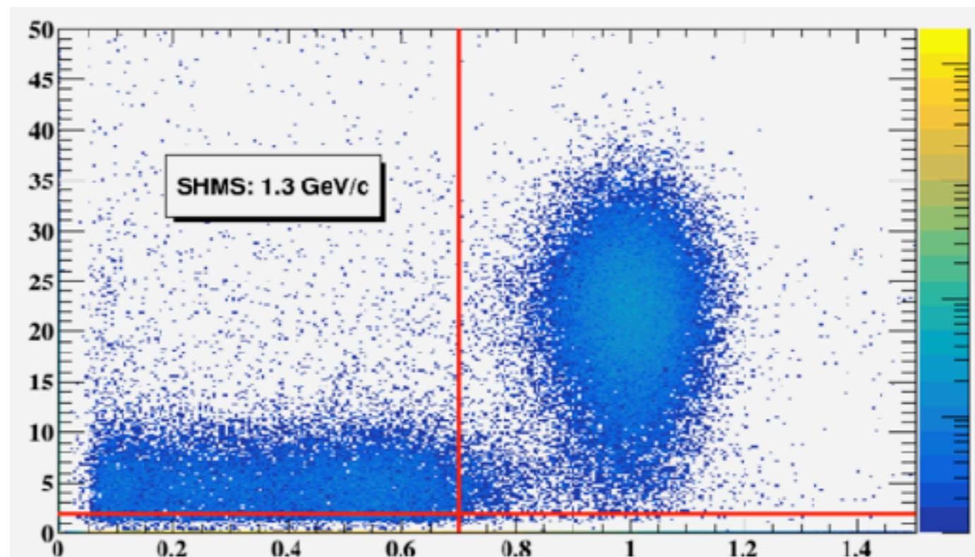
Energy Deposit in Calorimeter/Track Momentum
