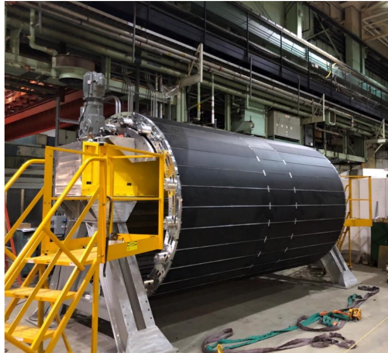
Inner Hcal barrel complete and ready to install EMC
