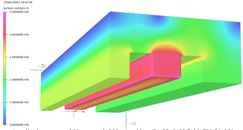
Arc dipole concept 380 cm steel, 399 cm with coils, 22 GeV field, TN-21-051. 120 cm remains for BPM, quad, corrector, bellows. Vacuum? Harp??
