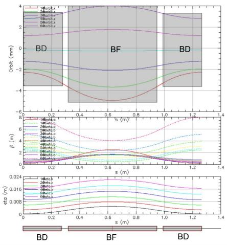
Large momentum acceptance FFA cell, configured with combined function magnets capable of transporting multiple energy beams through the same string of permanent magnets. BD horizontally diverging aka vertically focusing. BF horizontally focusing. Both also have dipole component. Very low dispersion (eta).
