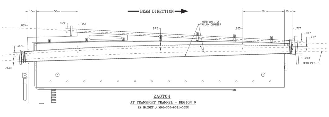
Third, fourth and fifth pass from top to bottom. Dimensions inches. A and C beams about 0.4" above/below B beam to reach correct holes in Lambertson in remaining drift. Exact locations needed to determine if plate thickness can be increased beyond 20 mm.
