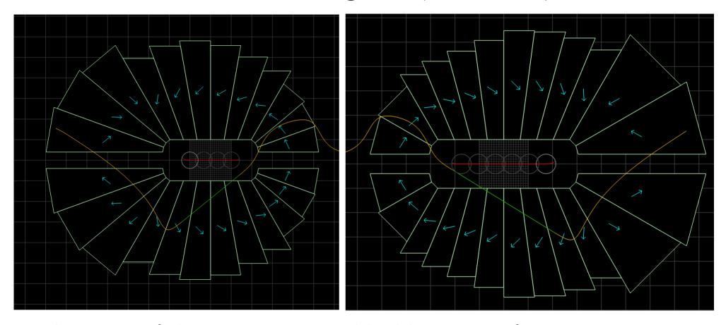
Left BD 105.8 cm<sup>2</sup> of permanent magnet material. Right BF 100.4 cm<sup>2</sup> Squares span 1 cm.
