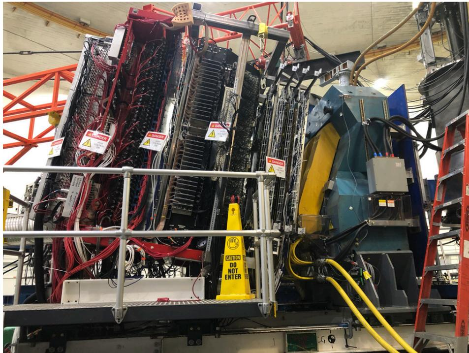
Cabling up the calorimeter, front end electronics, and DAQ in the hall
