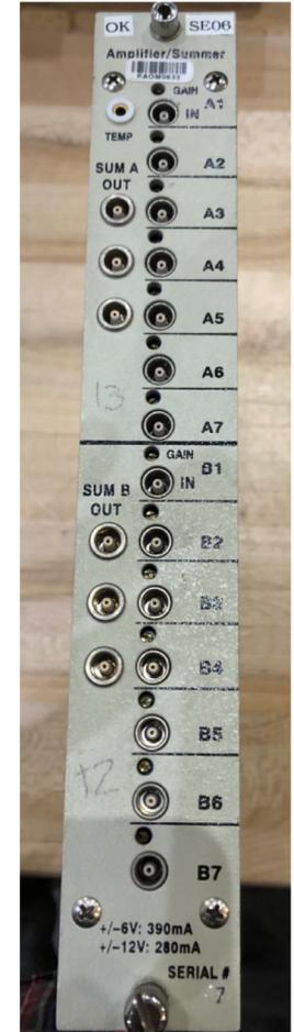
The outputs on the back of S/A modules saturate when the input crosses 200 mV
