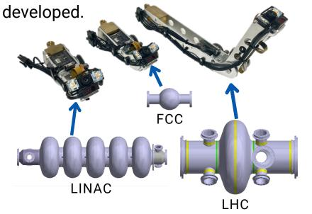
he three degrees of freedom robotic arm is equipped with many components which allow it to perform a safe cavity inspection.
