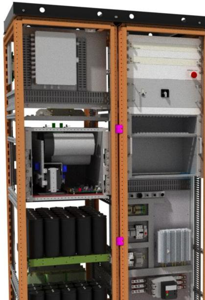
SIRIUS<sup>4</sup> (shown left) is a widely used CERN developed converter, capable of delivering ±450V and ± 200A, and is an example of a converter which has been emulated.
