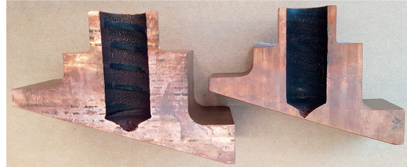
Cutaway of dipole photon shutter run until failure. Low conductivity water that cooled the absorber slowly eroded copper until a pinhole leak developed and water leaked into the vacuum space.
