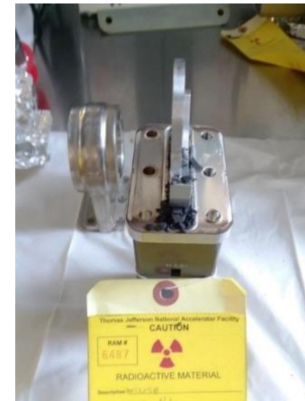
Radiation damaged C100 valve
