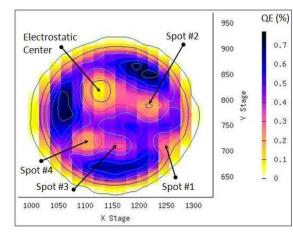
QE non-uniformity can be compensated to mitigate the associated effects by control of laser beam (intensity distribution & phase) This is where Al/ML may play a big role!
